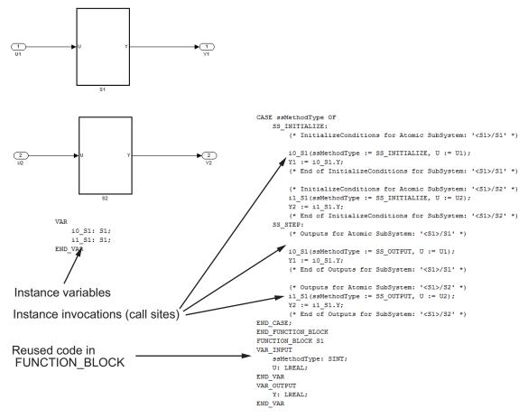
**4** Examine the generated Structured Text code. The code defines FUNCTION\_BLOCK ReusableSubsystem S1 once.
