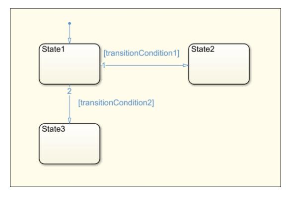
The state State1 is active as long transitionCondition1 and transitionCondition2 are not true. This means, State1 is active in one of these two cases:
