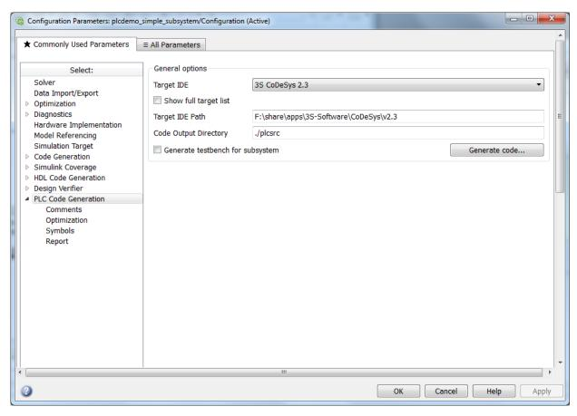
3 On the PLC Code Generation pane, select an option from the Target IDE list, for example, 3S CoDeSys 2.3.
