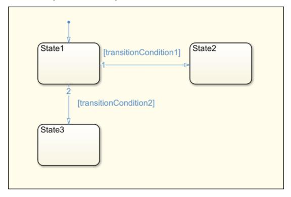
Some advanced Stateflow features are not supported because of inherent restrictions in Ladder Diagram semantics. You can use the function plccheckforladder to check if the chart has the required properties. You can also use the function plcprepareforladder to change certain chart properties so that the chart is ready for Ladder Diagram code generation.
