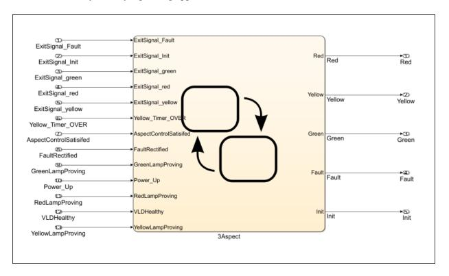
The chart consists of five states: Init, Fault, Red, Yellow, and Green. Based on the input to the chart, transitions to any of these states can take place. For instance, the state Red becomes active in the following scenarios:
