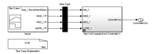
**c** Open the Inputs block in the test harness model. The Inputs block is a Signal Builder block that can have one or more signal groups.
