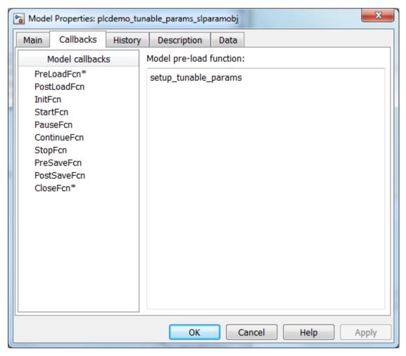
c On the Callbacks tab, select CloseFon. Enter clear K1 K2 K3; for Model close function.
