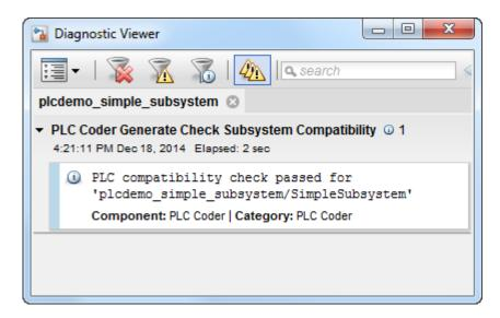
If the subsystem is not atomic, right-click the Subsystem block and select PLC Code, which prompts Enable "Treat as atomic unit" to generate code.
